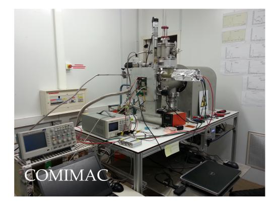
It is also now possible to plug the MIMAC pixelated anode/ electronics to the LHI for measuring higher energies (up to 100 keV) and heavy nuclear recoils (Ne, Ar, Xe !!)
