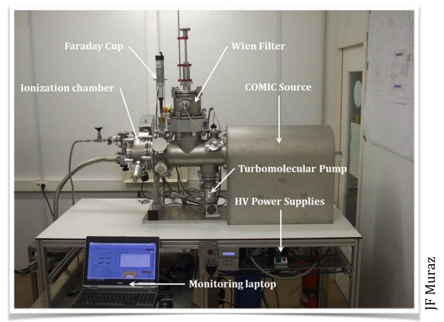
Primarily designed for \* the energy calibration of MIMAC up to ~50 keV
