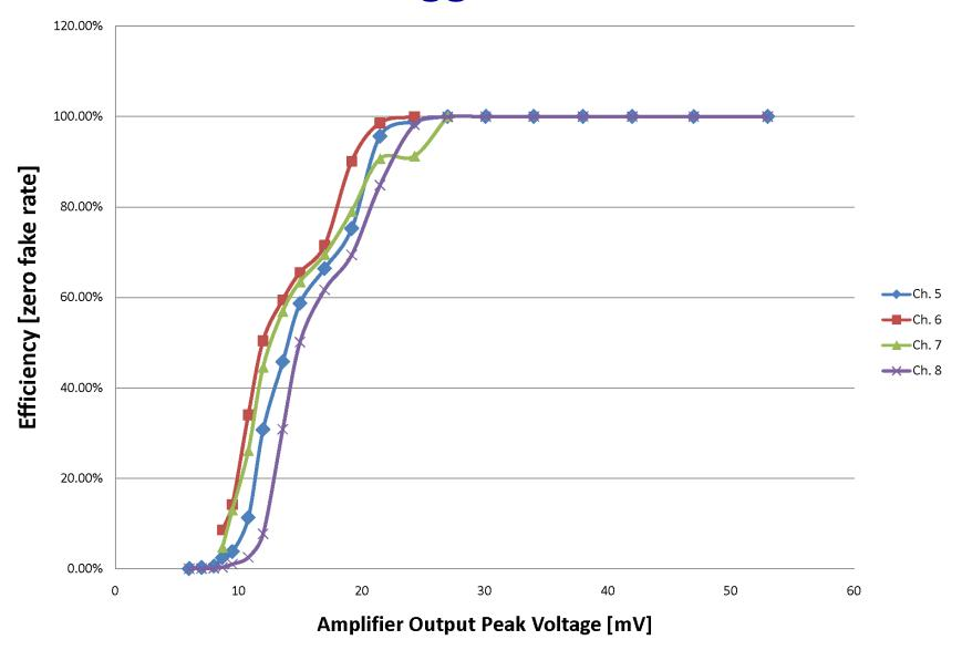
PMT-like output on test board: to be compared with laser data taken ("50mV" has trigger threshold cut off of about 15mV for real MCP signals)
