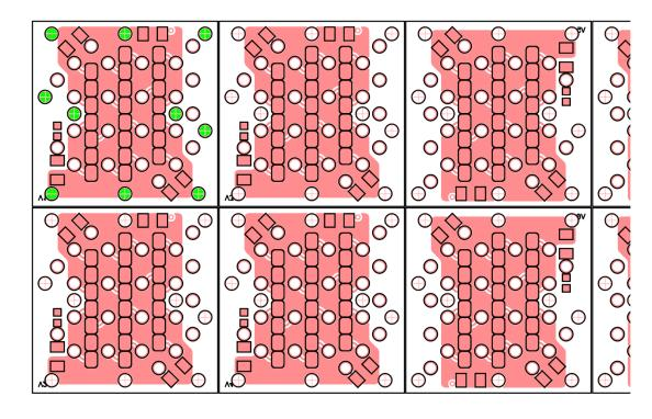
holes ~2 mm diameter, 4 at corners and 4 at middle of edges, pronounced satisfactory by Suzuki-san; "a few more in the middle would be good"
