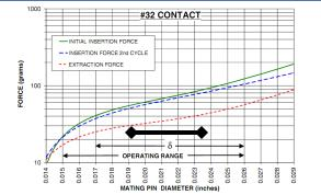
The insertion/extraction/normal force characteristics above were derived using 30 microinch gold plated contain and polished steel gauge pins having a bullet-shaped tip.
