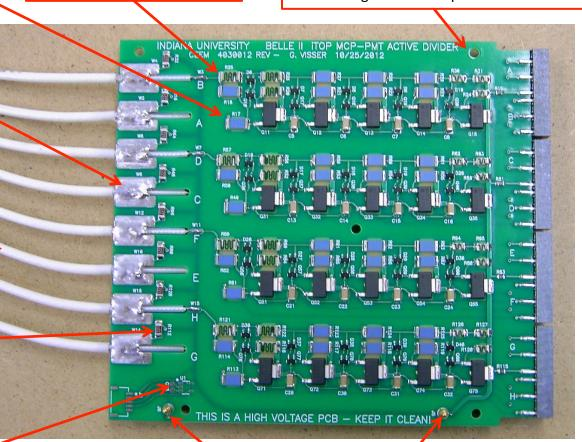
spring pin ground contacts (2 each top & bottom)
