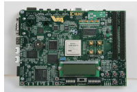
Figure 9: The Xilinx vertex V4 FPGA board
