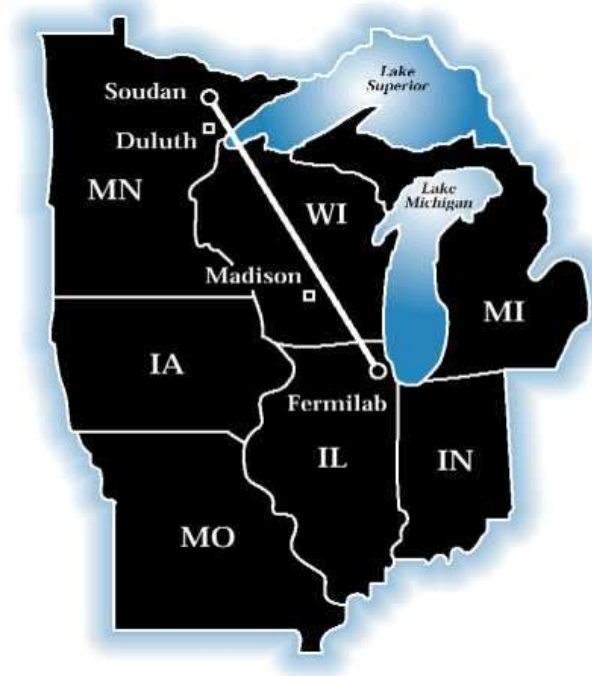
Two detectors: near detector at Fermilab ( L \sim 1\text{km} ), far detector at Soudan MN ( L \sim 735\text{km} )
