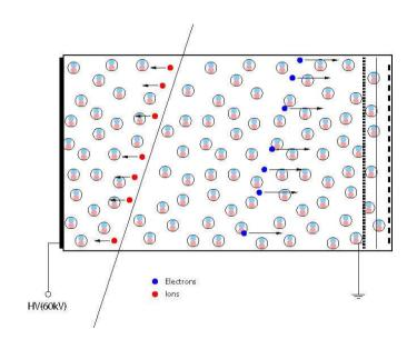
Drift ionization electrons over meters of pure liquid argon to collection planes to image track
