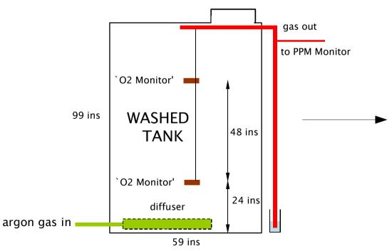
tank volume = 157 cftank cross section = 19 sfflow rate ~ 73.2 cf/h (reading for air was 86 scfh) climb rate ~ 3.8 f/h
