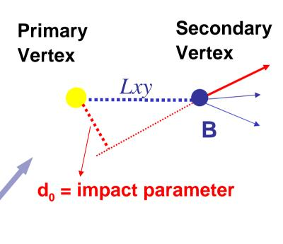
Silicon Vertex Trigger (SVT) – part of trigger system that finds displaced tracks and triggers on heavy flavor
