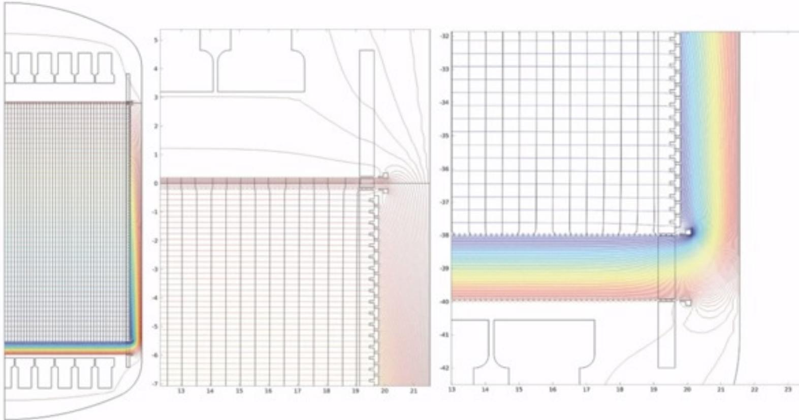
Uniformity in the drift region is key to position reconstruction and multiple scatter rejection, and fiducial volume definition
