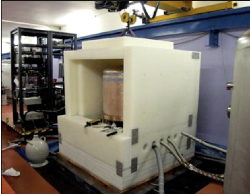
Hydrocarbon passive shielding to moderate external neutrons
