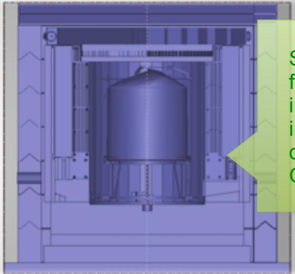
Snapshot of gdml part of the full ZEPLIN-III simulation – incl. shielding and detector in gdml – merged with detectors internals in GEANT 4 C++ code
