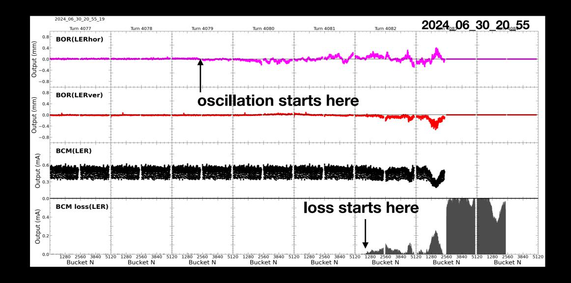
Beam oscillations typically begin a few turns before the actual beam loss. This early onset of oscillation provides an opportunity to diagnose the beam in advance.
