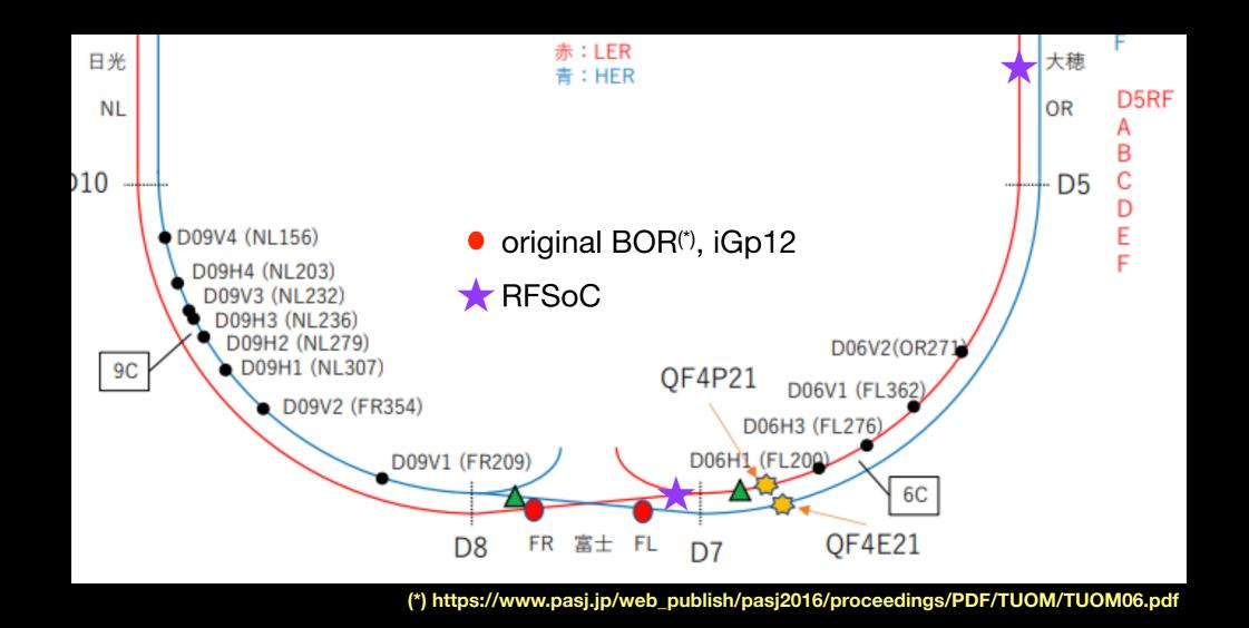
BOR, originally installed as a bunch feedback monitor, has proven to be very useful for SBL study. During LS1, additional BORs were added to futher monitor the beam.
