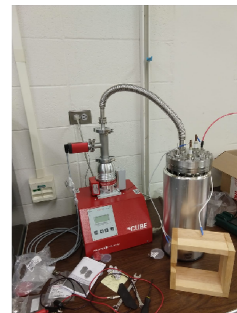
Vacuum pump and test chamber
