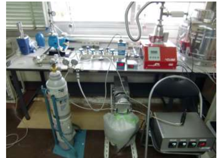
Filter for radon removal with zeolite
