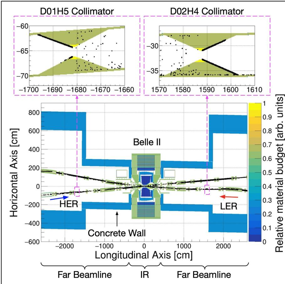
Recently improved Geant4 model of Belle II and collider cavern. Black dots represent single-beam losses 17
