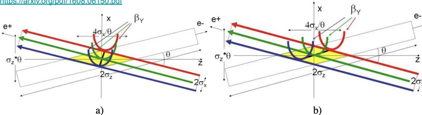
*Differently from the crab crossing scheme (KEKB) where bunches are tilted by the crab cavities with respect to the beam longitudinal axis, CW (SuperKEKB) rotates the optics function  $\beta_y$ .*
