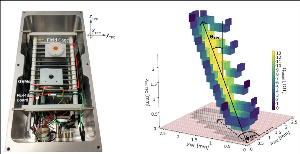
**Left:** Internal structure of the TPC. **Right:** Visualization of a nuclear recoil track reconstructed into 3D voxels.
