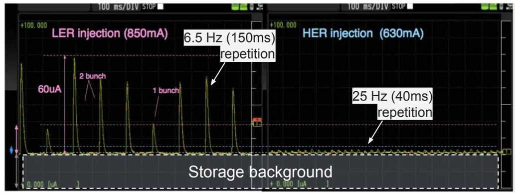
CDC leakage current during injection
