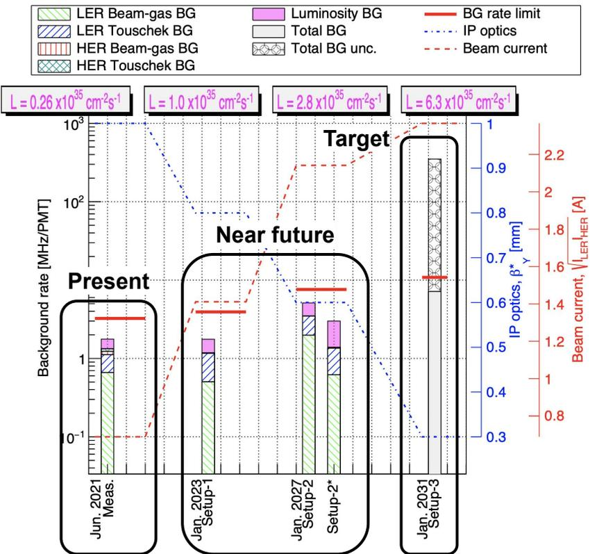
*Measured and predicted beam background hit rates in the Belle II TOP detector, for various machine configurations. These PMTs are expected to be the detector components most vulnerable to beam backgrounds.*
