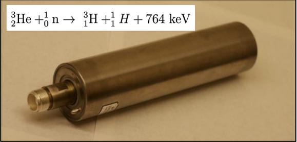
*Stainless steel tubes 24 cm long and 5 cm in diameter filled with  ${}^3\text{He}$  at 4 atm of pressure.*
