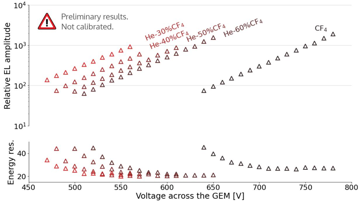
**Increasing the amount of CF<sub>4</sub> increases the EL(max) peak amplitude**, because the GEM sustains higher voltages before the onset of micro-discharges.
