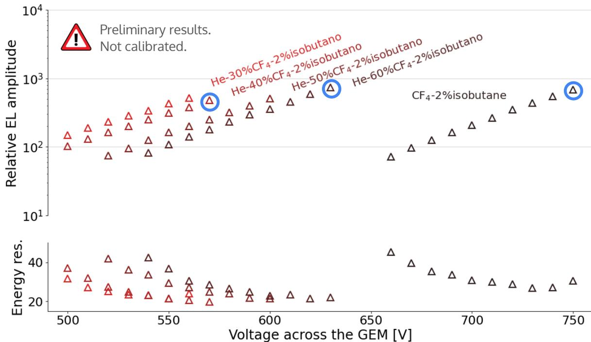
Increasing the amount of CF<sub>4</sub> in the mixture may **compensate** for the EL **quenching** due to the addition of **2% isobutane**.
