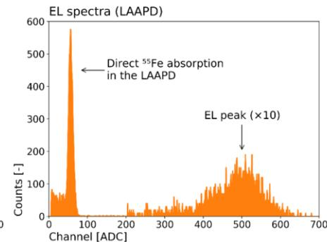
EL and  $^{55}\text{Fe}$  x-rays peak ratio
