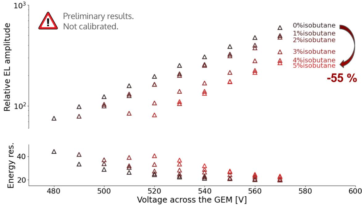
Isobutane seems to quench visible EL photons emitted by He-40%CF<sub>4</sub>: the EL peak amplitude decreases with increasing isobutane content.
