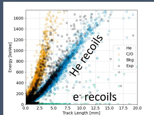
Figure 8: Reconstructed energy versus reconstructed length in simulated and experimental data in both TPCs before charge-loss corrections (top), after
