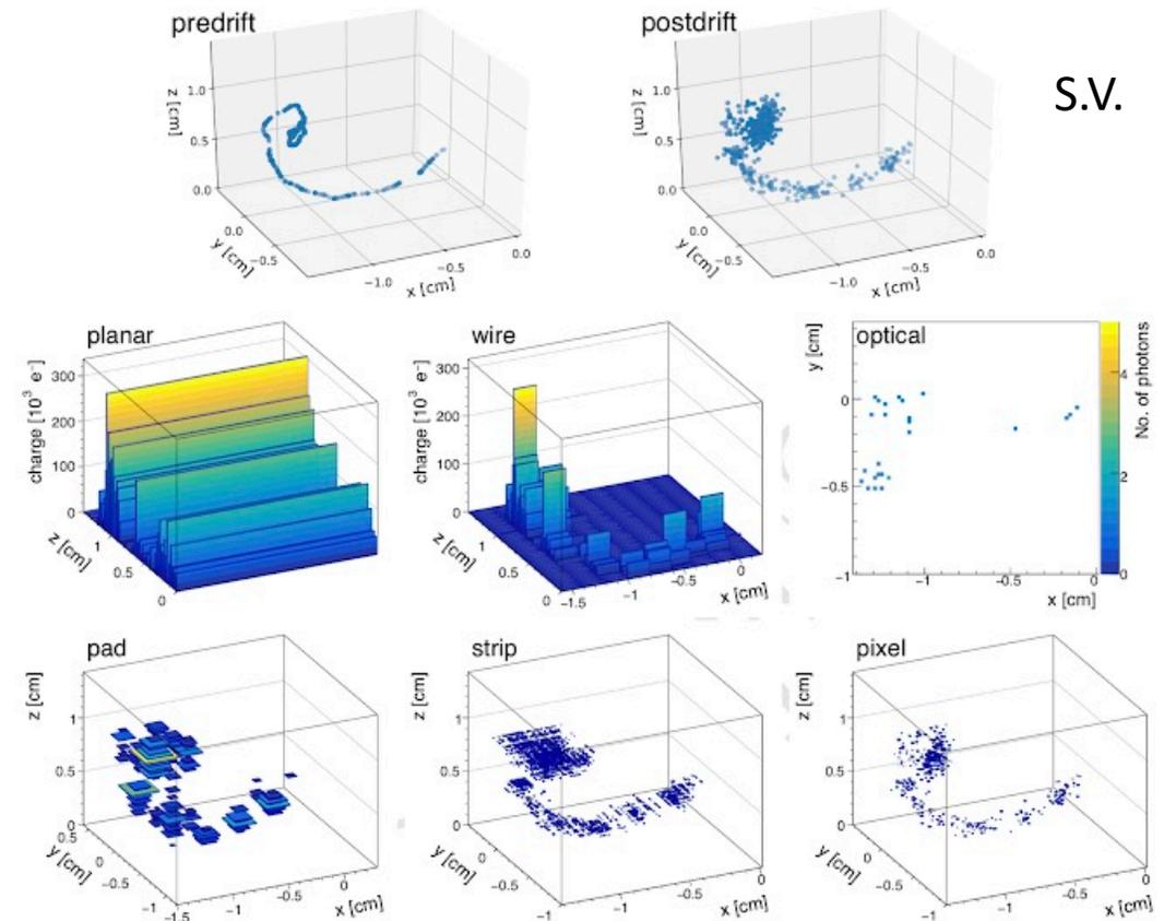
FIG. 10. Simulated 20 keV<sub>ee</sub> electron event in He:SF<sub>6</sub> gas before drift (top left), after 25 cm of drift (top right), and as measured by six readout technologies (remaining plots as labelled). Readout noise and threshold effects have been disabled.
