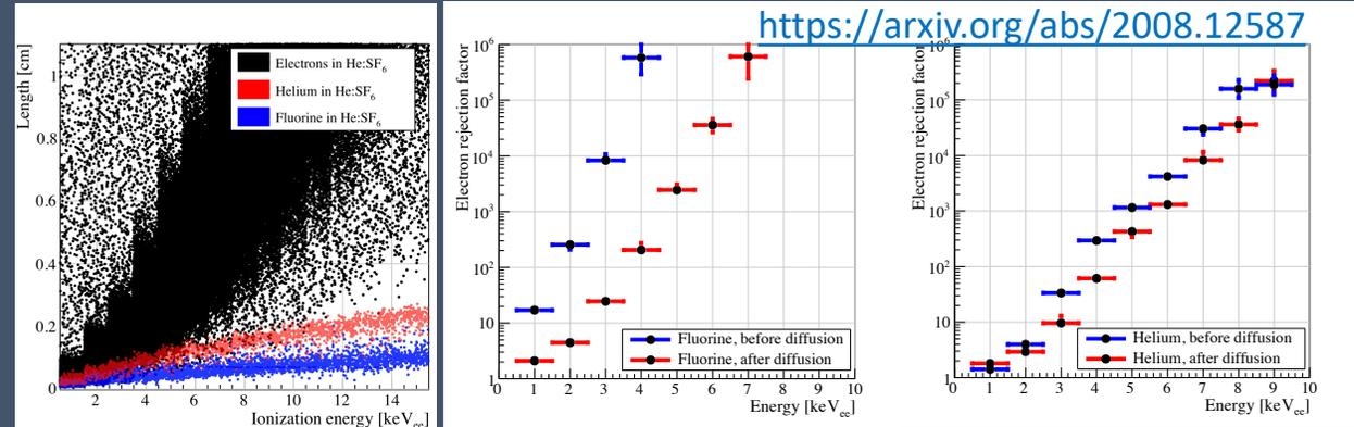
Electron rejection rises exponentially with ionization energy. When combined with flat bkg spectrum, will determine CYGNUS energy threshold for background free operation.
