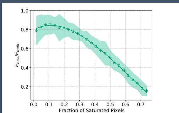
Figure 2: Ratio of reconstructed to true energy versus fraction of saturated pixels per event in all simulated recoils fit to a fourth-order polynomial. The shaded area represents one standard deviation of the data in each bin.
