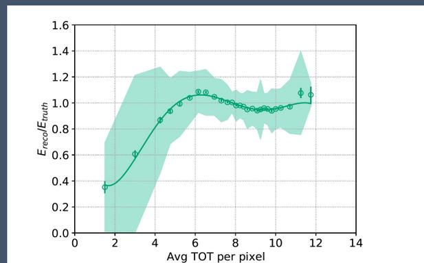
Figure 3: Ratio of reconstructed to true energy versus the average TOT in a single pixel per event fit to a fifth order polynomial. The shaded area represents one standard deviation of the data in each bin.
