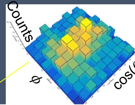
Measured directional neutron flux at TPC
