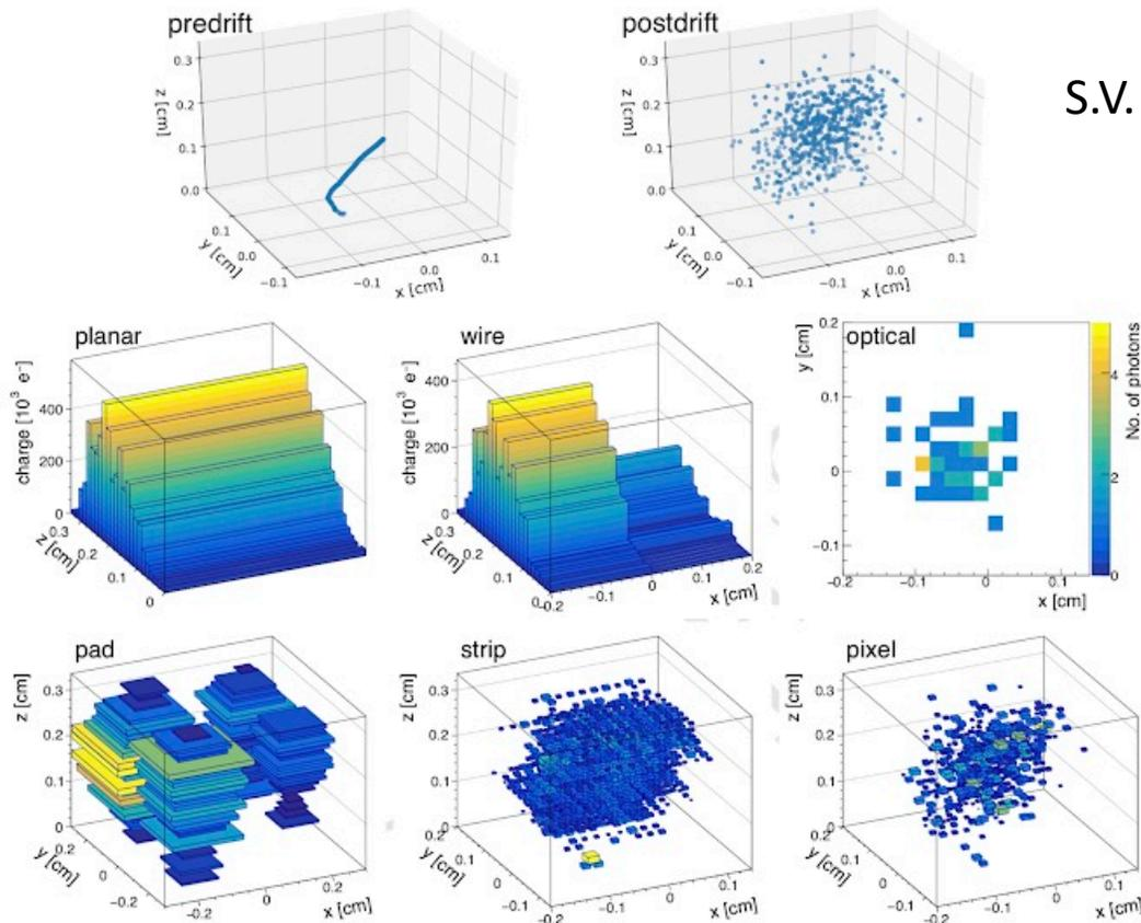
FIG. 9. Simulated 25 keV<sub>ee</sub> helium recoil event in He:SF<sub>6</sub> gas before drift (top left), after 25 cm of drift (top right), and as measured by six readout technologies (remaining plots as labelled). Readout noise and threshold effects have been disabled.
