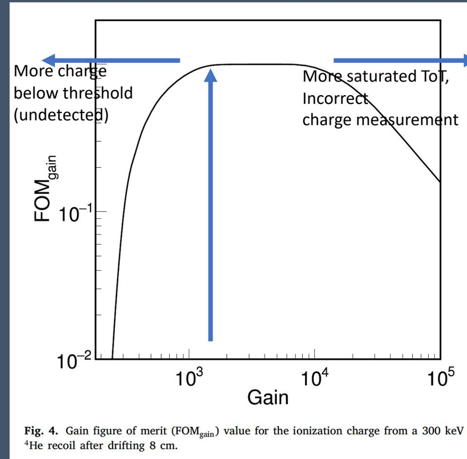
**Fig. 4.** Gain figure of merit (FOM<sub>gain</sub>) value for the ionization charge from a 300 keV <sup>4</sup>He recoil after drifting 8 cm.
