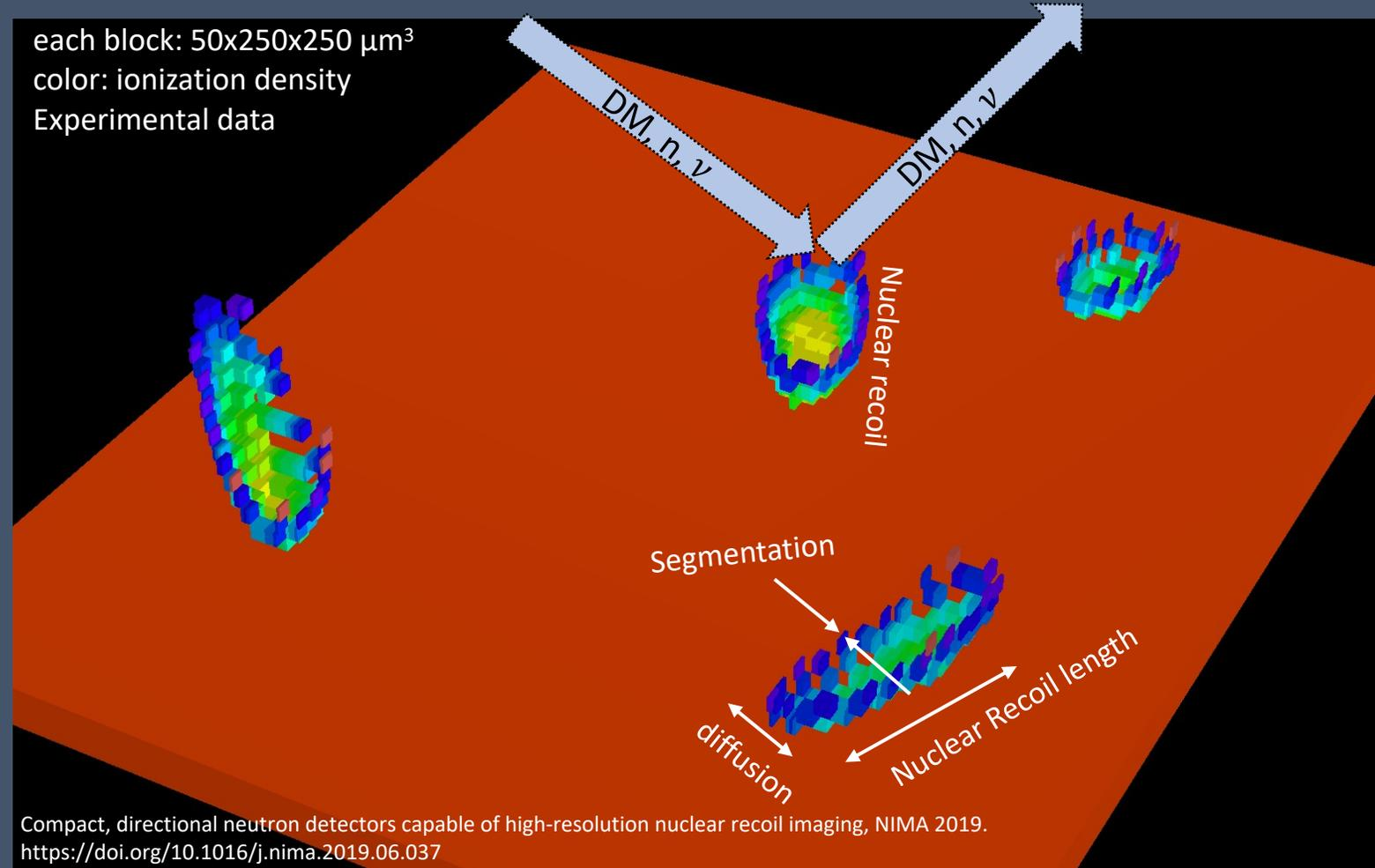
Want: segmentation (here:  $50 \times 250 \mu\text{m}$ ) < diffusion ( $\sim 200\text{-}500 \mu\text{m}$ ) < recoil length ( $\sim \text{mm}$ )
