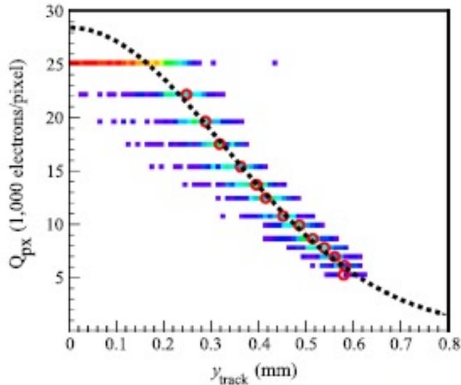
Fig. 3. Fit to the folded version of the corrected pixel charge ( $Q_{px}$ ) profile shown in Fig. 2 using the profile fit method described in Section 4.3. The Gaussian function (black dotted line) is fitted to the plot points (red open circles), which are placed at the mean  $Q$  and  $y_{track}$  positions for each unsaturated TOF layer. Error bars on the points are too small to show. (References to color apply to the web version of this article.)
