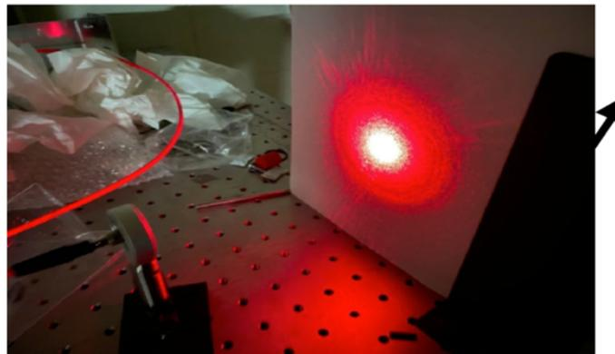
Testing light output from a fiber
