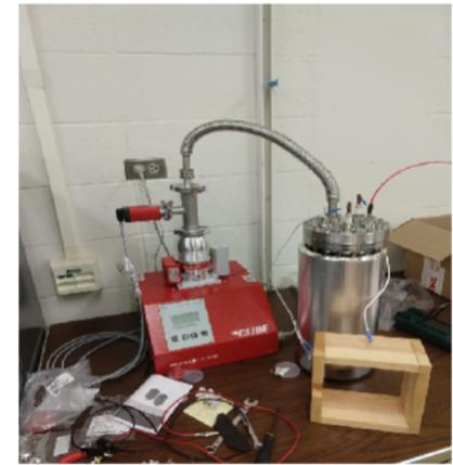
Vacuum pump and test chamber
