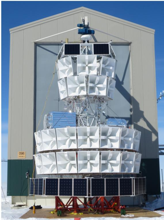
FIG. S1: The ANITA-IV payload in front of the LDB hangar, with lower photovoltaic panels deployed as in the flight configuration (C. Miki photo). Each of the quad-ridge horn antennas is about 0.95 m on a side.
