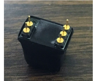
SiPM wrapped with scintillator by foil and black tape
