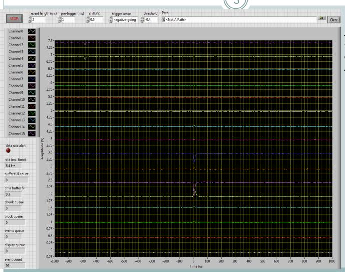
Note: in CF4, we see charge signals on all the channels.
