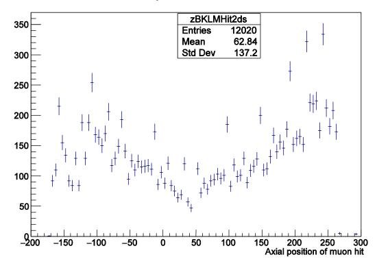
Description: The plot shows axial position of muon hit
